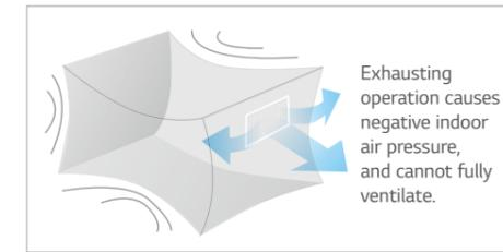
Exhausting and Supplying Simultaneously
